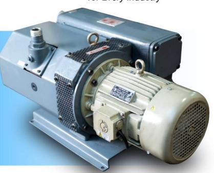
PVP series vacuum pumps are single-stage, oil-lubricated rotary vane pumps with oil re-circulation. Built for continuous operation under high intake pressures, they handle air and water vapour efficiently, ensuring reliable performance for industrial use, made from high-quality materials, PVP pumps combine durability with economical operation.
